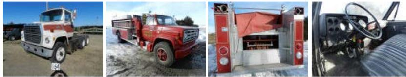
1985 GMC pumper truck, 427 engine, Allison automatic trans., w/750 gal. tank & Ford engine w/ 6" pump, low miles, pumps 720 gal. per minute
