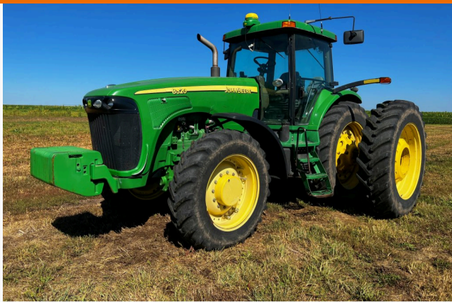
2007 John Deere 8230 MFWD Tractor, 4,834 hrs., rear wheel wts & spacers, 4 hyd., large 1000 PTO, hyd. 3rd length, 16 front weights, 480/80R46 rear dual tires, 380/85R34 front tires, SN: RW82300P15880
