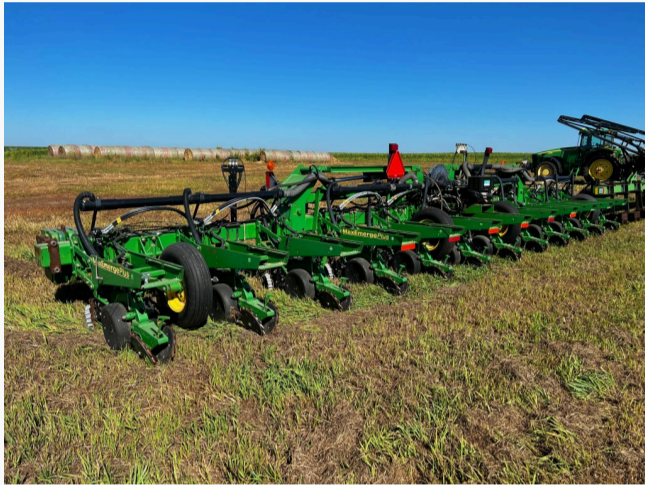
John Deere MaxEmerge Plus 12R36 Planter, Clean Sweep Yetter furrow openers with pneumatic pressure, compressor and monitor, Delta Force Precision Planting w/hyd. down force, Precision meters & boxes, SureFire fertilizer pumps w/dual 12V electric & flow meter, Keeton in-furrow seed firmers, stabilizer wheels, large seed boxes, markers & Lofquist closing wheels
